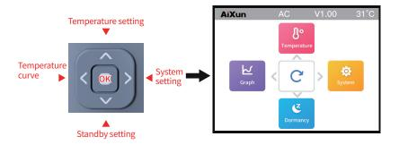
The power on interface of the station default to be the main interface. Click the middle function button to enter the function setting interface. The functions displayed on the interface correspond to the function buttons one by one, a nd the user can operate according to the prompts.
